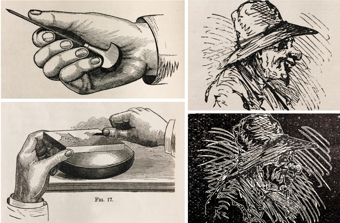
Figure 6. The Engraver's Hands and His First Cuts, from Manual of Wood Engraving for the Amateur , Arthur Hope, 1882. The illustrations show how the engraver holds the tool in his palm (top left) and how, for support, the thumb rested on the wood while cutting. The engraver given an image on the wood (top right) would begin by cutting around each line (bottom right).
